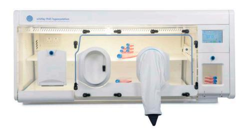
eliminates cellular stress linked to variations in temperature, pH levels and oxidation – resulting in better cell lines. The Whitley Instant Access Port and has a 440 litre capacity. The 12 litre airlock will accommodate a variety of pipettes, culture
