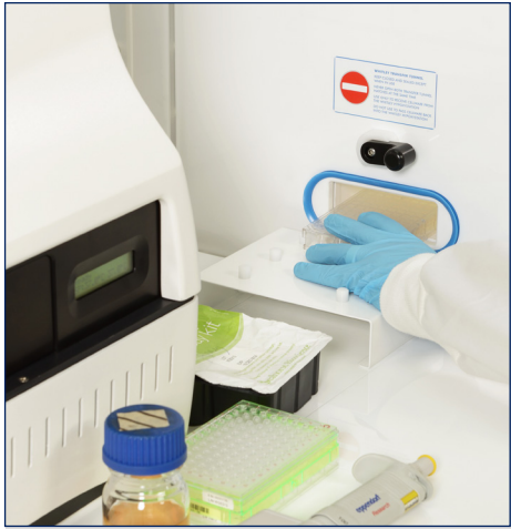
Tunnel de Transfert
