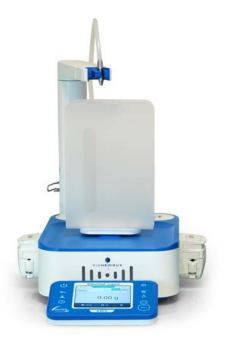
Dilumats save time and money by automating the laborious process of making and standardising the initial sample dilution. There is no longer a need for you to spend time and effort weighing out exact amounts of sample - the Dilumat can receive any sample volume and dilute as required.
