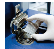
Insert target plate into MALDI-TOF; start run.
