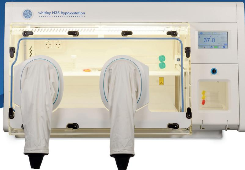
The Whitley Hypoxystation creates physiological cell culture conditions with regard to temperature, humidity and gas atmosphere. The uniquely low gas consumption ( $N_2$  and  $CO_2$ ) of a Hypoxystation is significant because:
