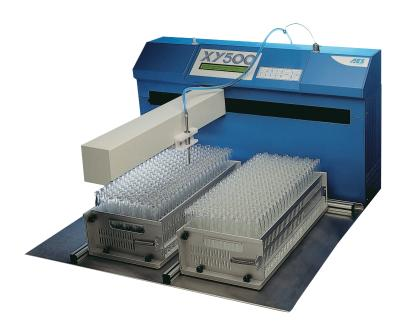
The XY500 automates the manual process of filling vessels with a predetermined quantity of liquid such as broth, sterile water, diluent and culture media. It comes complete with an adjustable 252 tube rack and a dispensing nozzle.
